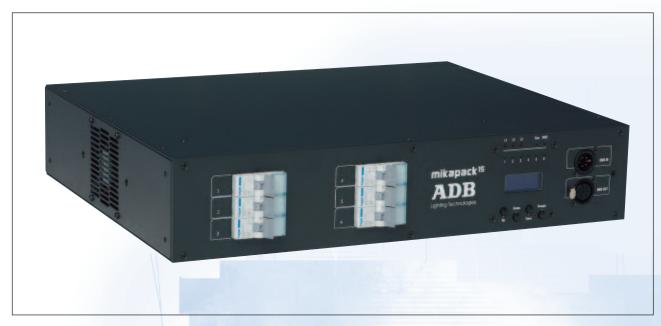
6 x 3 kW all-digital dimmer pack for 19" rack mounting combining high quality with low cost and above average performance, for general purpose applications in stage and architectural lighting whenever space, cost and reliability are the prime considerations.
